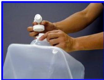
1. Put the stopcock to a "cubic container for cleaning".
