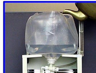
3. Pour hot water (under 70 ) approx 5 liters into the "cubic container for cleaning".
