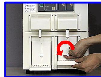
6. After all hot water comes out, replace the server bottle holder and take off the "cubic container for cleaning".
