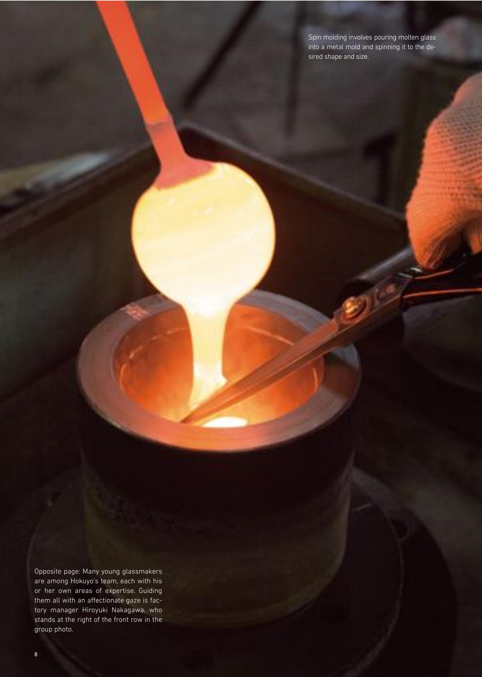
Spin molding involves pouring molten glass into a metal mold and spinning it to the desired shape and size.
